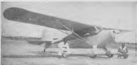
The Aruba Flying Club's inventory of planes increased to six this month with the four-engine arrival of this new Avanca "Chief", a side-by-side two seater. It was a wheel instead of a stick, first of this type here, and the manual controls have to be handled with the left hand. That's mechanic Miguel Felipe at left and Hamilton Blair at right, who helped assemble the ship.
